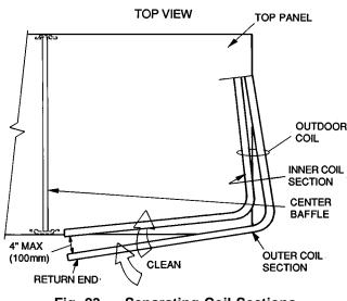
Fig. 23 — Separating Coil Sections
